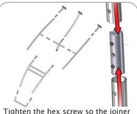
Tighten the hex screw so the joiner seperates and tightens against the inside of the tubing, locking the joiner and tubing together.
