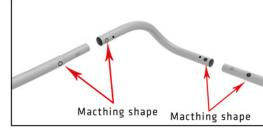
Assemble the two long curved and long straight sections (Connected with bungee cord). The frame is symmetrical. Either curved pole can be top or bottom.
